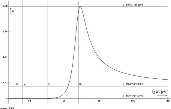
Figure 134 Correction factor  $\alpha$  as a function of the energy of the electron
