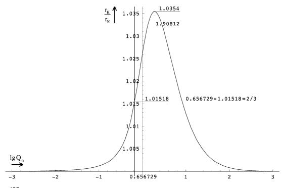
Figure 125 Ratio between the length of the constant wave-count vector  $r\kappa$  and the length of the zero vector  $r\aleph$  as a function of  $Q_0$
