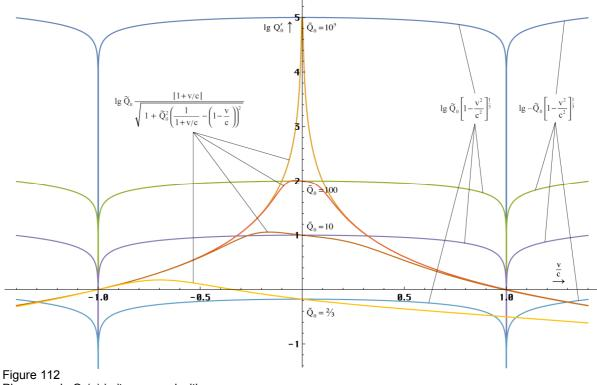
Phase angle  $Q_0(v)$  in its own and with respect to another frame of reference
