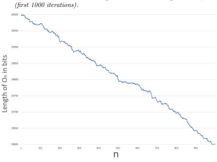
FIGURE 4. Decrease of  $O_n$  length for 20000 bits long initial  $X_0$  (first 1000 iterations).
