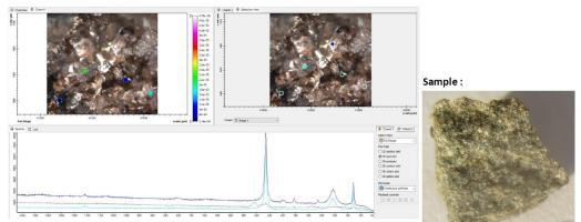
Indication for a shock event are the shifts of the marked Quartz spectral lines towards 463 and 204
