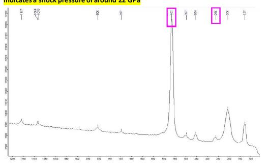
Indication for a shock event is the shift of the marked Quartz spectral line towards 205
