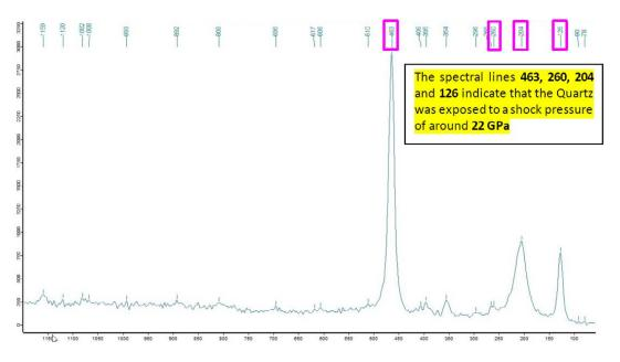
Indication for a shock event are the shifts of the marked Quartz spectral lines towards 463 and 126
