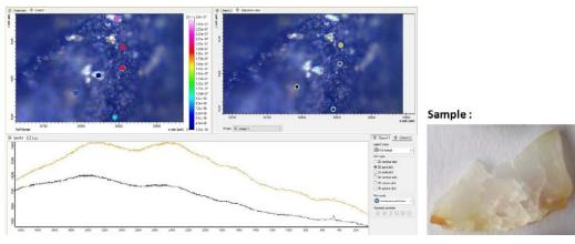
Indication for a shock event are the shifts of the marked Quartz spectral lines towards 463, 260 and 205
