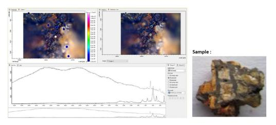
Indication for a shock event are the shifts of the marked Quartz spectral lines towards 463, 260 and 204
