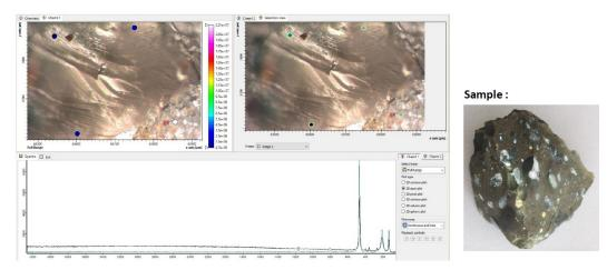
Indication for a shock event are the shifts of the marked Quartz spectral lines towards 263 and 205
