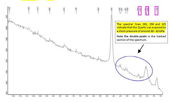
Indication for a shock event are the shifts of the marked Quartz spectral lines towards 260 and 205
