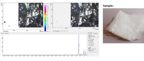
The spectral lines 463, 260 and 205 indicate that the Quartz was exposed to a shock pressure of 22 GPa
