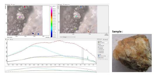
Indication for a shock event are the shifts of the marked Quartz spectral lines towards 463, 262 and 205
