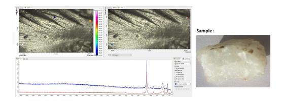
Indication for a shock event are the shifts of the marked Quartz spectral lines towards 204 and 124
