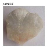
The spectral lines 463, 261, 204 and 126 indicate that the Quartz was exposed to a shock pressure of ≈ 22 GPa
