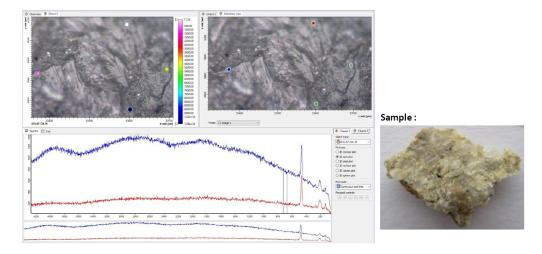
Indication for a shock event are the shifts of the marked Quartz spectral lines towards 261, 204 and 125
