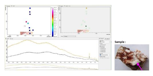
Indication for a shock event are the shifts of the marked Quartz spectral lines towards 463, 261, 203 and 126
