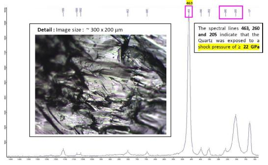
The spectral lines 463, 261, 205 and 125 indicate that the Quartz was exposed to a shock pressure of  $\approx$  22 GPa!
