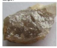
The spectral lines 463, 258/264, 205 and 126 indicate that the Quartz was exposed to a shock pressure of around 22 GPa!
