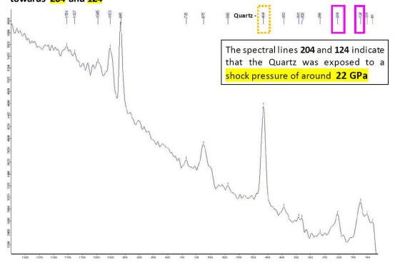
Indication for a shock event are the shifts of the marked Quartz spectral lines towards 263 and 205
