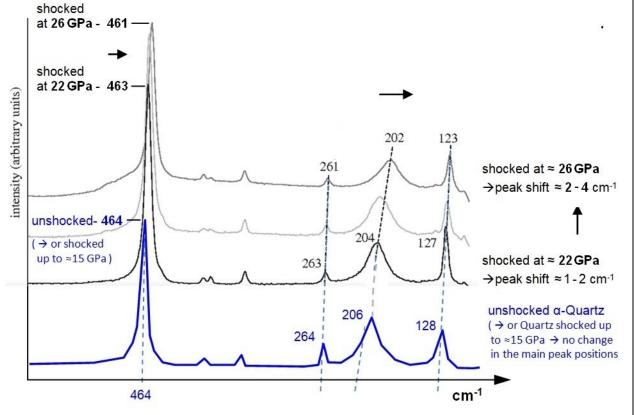
Quartz shocked with 22 GPa and 26 GPA  $\rightarrow$  shows shifts of the main RAMAN-peaks of 1 - 4 cm<sup>-1</sup> towards lower frequencies, compared with unshocked Quartz
