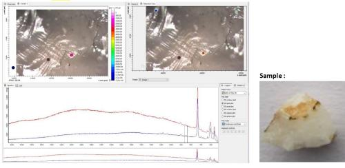
Indication for a shock event are the shifts of the marked Quartz spectral lines towards 463, 261 and 205
