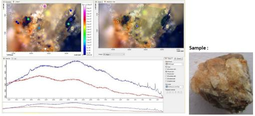
Indication for a shock event are the shifts of the marked Quartz spectral lines towards 463, 261, 198 and 125
