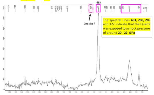
Indication for a shock event is the shift of the marked main Quartz spectral line towards 463
