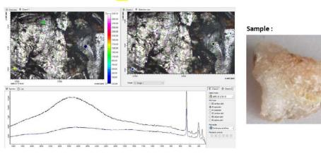
The spectral lines 463, 262/268 and 125 indicate that the Quartz was exposed to a shock pressure of ≈ 22 GPa
