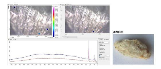
The shift of the main spectral line of Quartz towards 463 in the sample indicates a shock pressure of around 22 GPa
