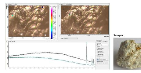
Indication for a shock event are the shifts of the marked Quartz spectral lines towards 261 and 201 (209)
