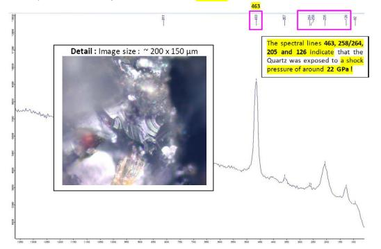
The spectral lines 263 and 126 indicate that the Quartz was exposed to a shock pressure of around 22 GPa!
