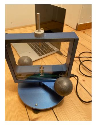
**Figure 1:** Low-budget modern Cavendish apparatus combining old mechanics with modern electronics that feed directly to your computer through a USB cable. It is remarkable that, in using such an instrument, we can measure the Planck mass with only about 5% error.
