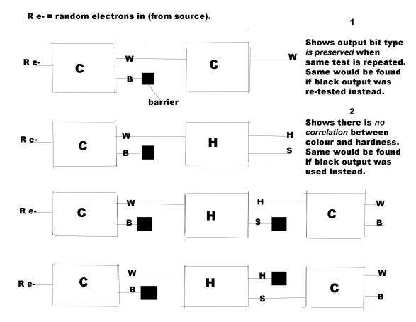
3 The last two tests sequences shown indicate that the sole output bit type is not preserved after exposure to a different test (orientation of apparataus).
