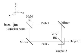
FIG. 1. Schematic view of Mach-Zehnder Interferometer (MZI). BS:Beam Splitter.
