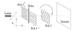
FIG. 3. Typical setup for the Quantum Eraser. Pol1 and Pol2 are fixed linear polarizers with polarizing axes perpendicular (x and y). Pol3 is a revolvable linear polarizer. <sup>2,39</sup>
