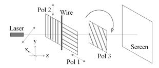
FIG. 3. Typical setup for the Quantum Eraser. Pol1 and Pol2 are fixed linear polarizers with polarizing axes perpendicular (x and y). Pol3 is a revolvable linear polarizer. <sup>2,38</sup>
