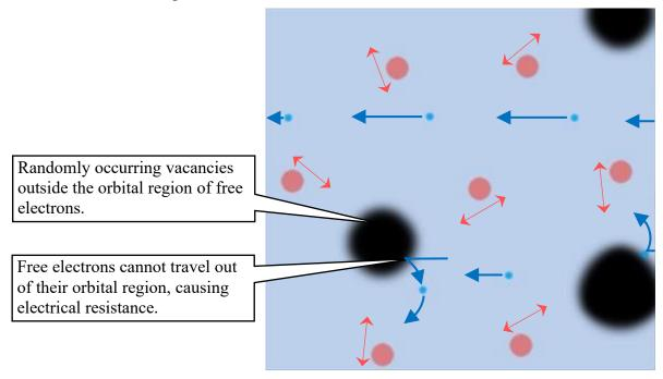
This proposition explains the phenomenon wherein as temperature decreases, the normal conductivity suddenly transitions to superconductivity with zero electrical resistance at the Tc.
