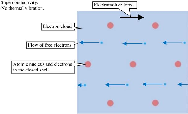
Superconductivity. Thermal vibration at temperatures below the superconducting transition temperature (Tc).
