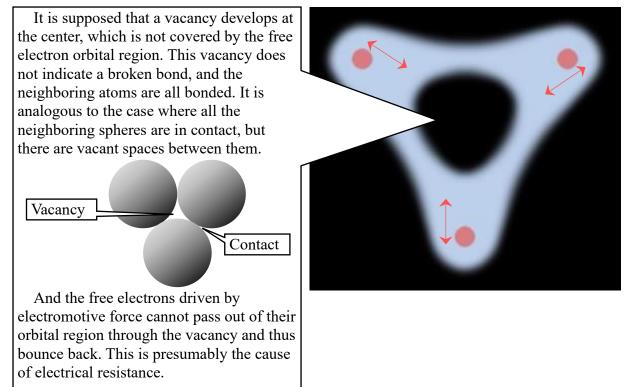
Free electrons flowing in a conductor by the electromotive force.
