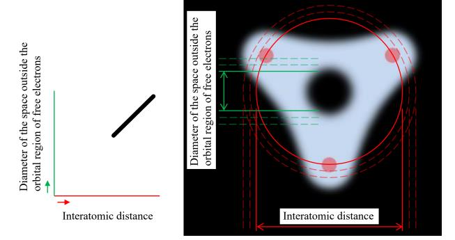
At a certain point as the interatomic distance decreases, the space outside the free electron orbital region suddenly shrinks due to the adhesive property of the electron cloud bond. In other words, when the thermal amplitude drops to a certain degree, the randomly occurring spaces outside the free electron orbital region suddenly shrinks and will not occur. This theory suggests that the electrical resistance suddenly becomes zero at the Tc.
