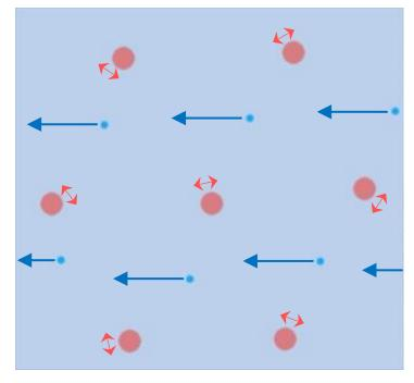
Normal conduction. Thermal vibration at temperatures above the Tc.
