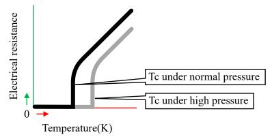
Under high pressures, even for the thermal vibration with the same amplitude, vacant regions between the free electron orbital regions occur less frequently due to the reduced interatomic distance. Therefore, the Tc rises.
