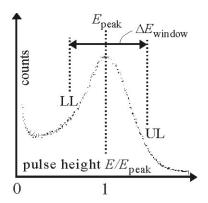
Figure 1. PMT pulse-height response
