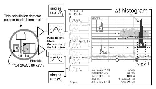
Figure 3.  $\gamma$ -ray experiment in tandem geometry using  $^{109}$ Cd. DSO screen is annotated.
