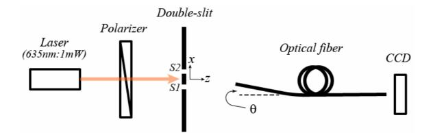
Fig. 1 Apparatus to observe interference fringes using an optical fiber. The laser beam passes through a polarizing plate (45 degrees) and a double-slit to form interference fringes. The interfering light enters an optical fiber (inclination  $\theta$ ) and is measured by a CCD placed at the end. The optical fiber is scanned in the *x* and *z* directions by motorized stages to obtain an intensity distribution.
