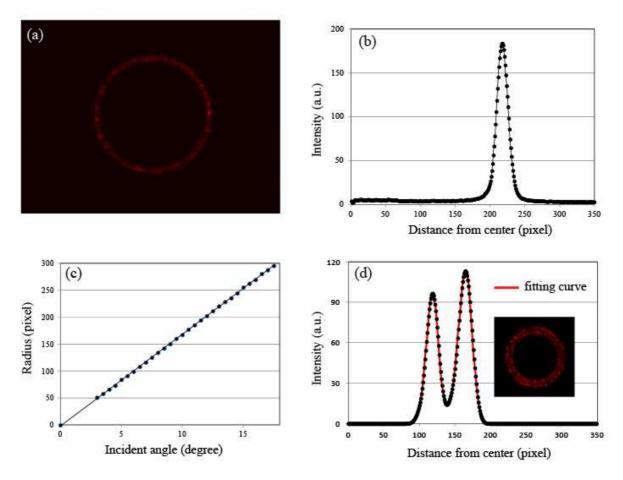
Fig. 5 Observation of photon movement using an MMF. (a) Image of a circle at the exit surface of the fiber when light entered the fiber obliquely, (b) the intensity distribution with respect to the distance from the center of the circle, (c) the correlation between the incident angle and the radius of the circle, and (d) the intensity distribution when light waves entered from two directions.
