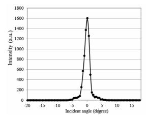
Fig. 2 Correlation of the incident angle and transmitted light of a single-mode optical fiber.
