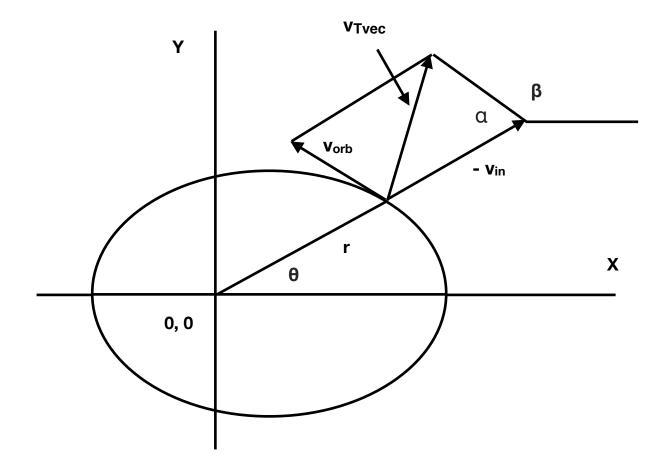
Figure D.1 Elliptical Orbit of GPS Satellite - Ellipticity Exaggerated
