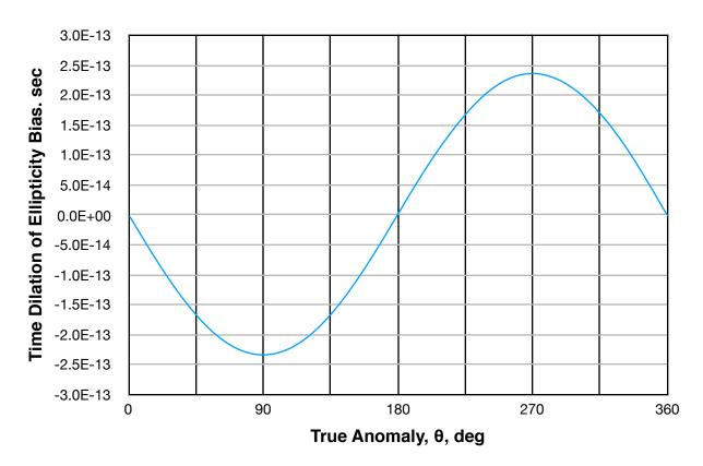
Figure 1. Time Dilation Difference, Vector Minus Algebraic Calculation with Ellipticity of 0.001
