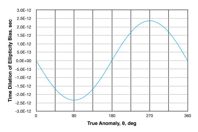
Figure 2. Time Dilation Difference, Vector Minus Algebraic Calculation with Ellipticity of 0.01
