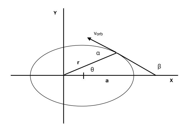
Figure B.1 Elliptical Orbit Parameters Eccentricity Exaggerated
