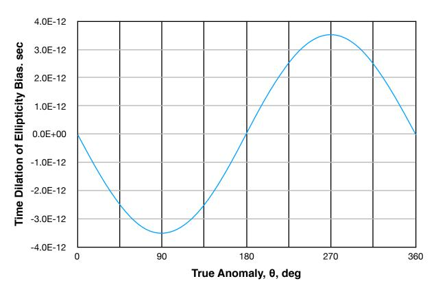
Figure 3. Time Dilation Difference, Vector Minus Algebraic Calculation with Ellipticity of 0.015
