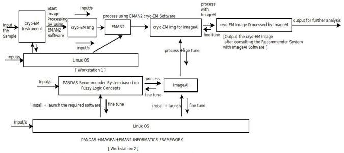
SIMPLE ALGORITHM FOR ADVANCED IMAGE PROCESSING USING PYTHON
