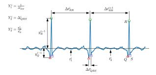
**FIGURE 3**. Statistical ECG features of interest extracted from the sensor ECG signal
