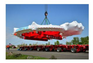
Fig. 9: Transportation of the 600 ton magnet to Fermilab
