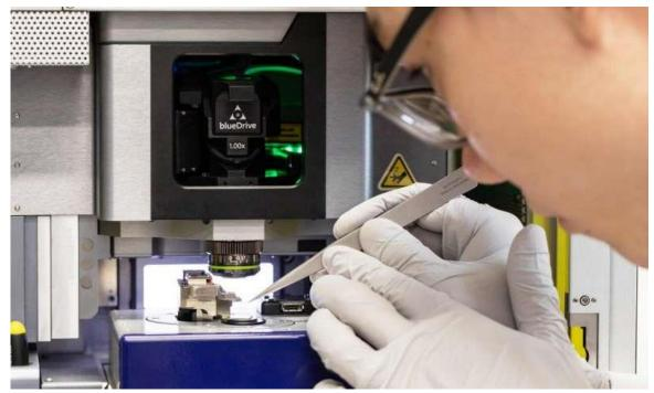
University of Toronto Engineering researchers used an atomic force microscope (pictured) to measure the ability of graphene to resist mechanical fatigue. They found that the material can
