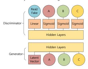
Fig1. AC-GAN that trains A, B, and C conditions
