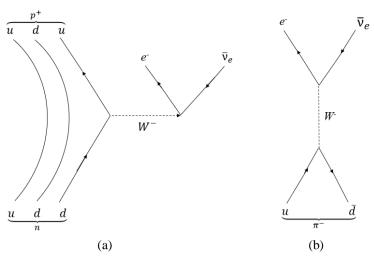
Figure 1. (a) The neutron decay through the weak interaction [1,2]. (b) The negative pion decay in the weak interaction [1,2].
