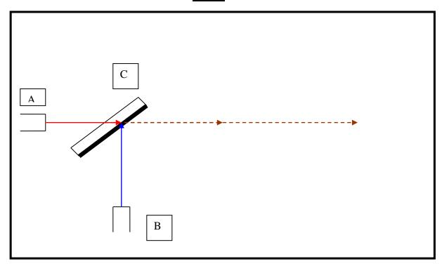
An Electromagnetic Wave source A generates a much focused one dimensional electromagnetic traveling wave (red), that passes through a half transparent mirror C, and continues to travel, as indicated by the dotted line. Another Electromagnetic Wave source B generates a much focused, one dimensional electromagnetic traveling wave (blue), that is deflected by the mirror C, such that it continues to travel on exactly the same line as the first wave A, as indicated by the dotted line.
