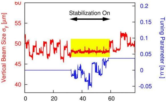
This chart shows how vertical beam-size stability greatly improves when a neural network is implemented during Advanced Light Source operations. When the so-called "feed-forward" correction is implemented, the fluctuations in the vertical beam size are stabilized down to the subpercent level (see yellow-highlighted section) from levels that otherwise range to several percent. Credit: Lawrence Berkeley National Laboratory
