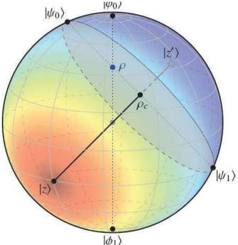
Entanglement on a sphere: This Bloch sphere shows entanglement for the one-root state  $\rho$  and its radial state  $\rho$ c. The color on the sphere corresponds to the value of the entanglement, which is determined by the distance from the root state z, the point at which there is no entanglement. The
