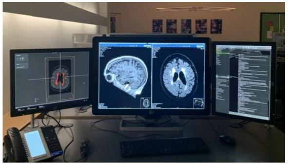
Here, the IMAGR interface (left monitor) shows the results of the white-matter hyperintensity detection and quantification algorithm. The middle monitor shows the PACS interface. The right monitor shows the electronic health record. (Courtesy: Olivier Middendorp – NRC)
