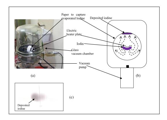
**Fig. 1.** Figure extracted from the reference [2] - Experimental set-up to observe movement of heat-evaporated iodine vapor in vacuum.
