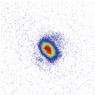
A mixture of two ultracold gases that attract each other can form an ultra-dilute liquid, which remains self-bound in a droplet even in the absence of any confinement. Credit: ICFO
