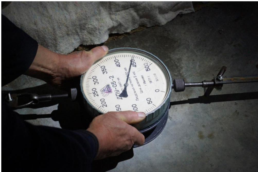
Fig. 8. Photo of the measurement showing magnitude of the pulse thrust force F_T of 450 kgf generated by KVD-1-2009
