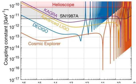
This chart compares the sensitivity of gravitational-wave detectors suitable for the axion hunt. The project is ongoing at the University of Tokyo Institute for Cosmic Ray Research. Credit: Nagano et al
