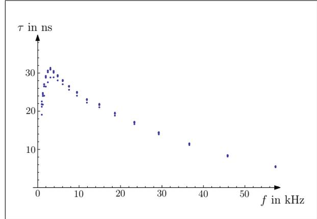
Figure 1: Measured phase error between inputs A and B of the oscilloscope depending on the signal frequency  $f$
