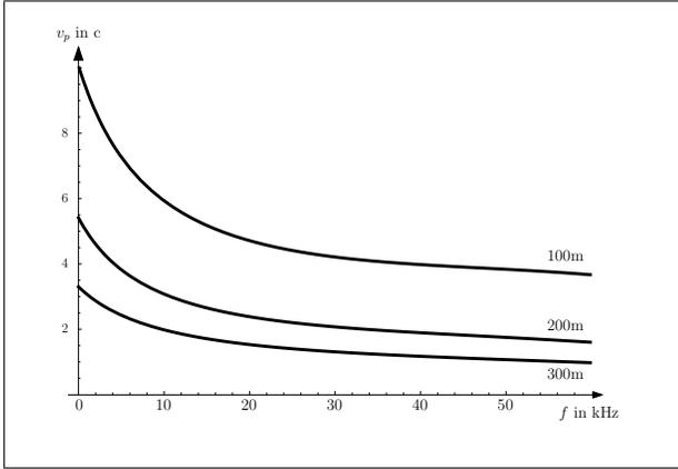
Figure 3: Phase velocities  $v_p$  as a function of cable length and signal frequency  $f$
