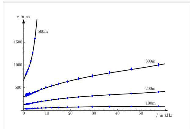
Figure 2: Measured signal delays  $\tau$  between the two channels for sine waves as a function of cable length and signal frequency  $f$
