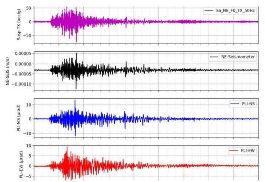
The PLI (bottom two plots) picked up the same signals as devices already installed at Virgo (top two plots) for an earthquake in Northern Italy on 17 August. Credit: Beniamino Di Girolamo/CERN
