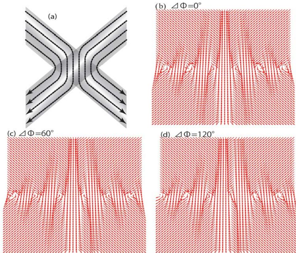
Fig. 1. (a) Schematic view of the Bohmian trajectories of photons in the crossed beams incident from the  $\pm 45^\circ$  direction. (b, c, d) Vector diagrams (ignoring magnitude) of Bohmian orbit obtained by simulation near the center of the crossed beams. The phase difference between left and right beams was 0, 60, and 120 degrees, respectively.
