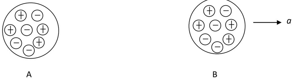
Assume that force is applied to physical object B to accelerate it away from body A. If we make the conventional assumption that the interaction between opposite charges is equal in magnitude to the interaction between similar charges, the fourth component of Weber's formula would not predict inertia for neutral bodies.
