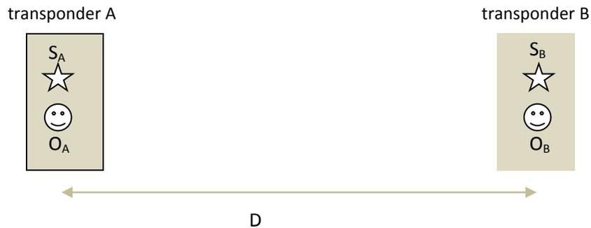
Initially  $S_A$  emits a short light pulse, which will be detected by  $O_B$ , which will trigger  $S_B$  to immediately emit a short light pulse, which will be detected by  $O_A$ , which will trigger  $S_A$  to immediately emit a short light pulse, which will be detected by  $O_B$ , and so on. An electronic counter counts the number of pulses in a given period of time.
