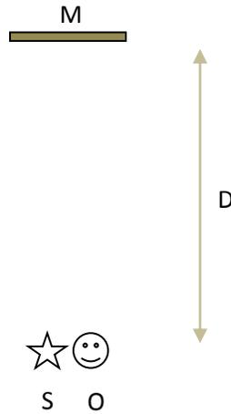
Initially, a short light pulse is emitted by the source S, which will travel to mirror M, and reflected back to the detector O. Upon detecting the light pulse, detector O immediately triggers source S to emit a short light pulse again, which will travel to the mirror, reflected back and detected by O, which triggers source S and so on. A counter counts the number of pulses emitted. If we don't consider the finite time delay between detection and re-emission, the round trip time will be:
