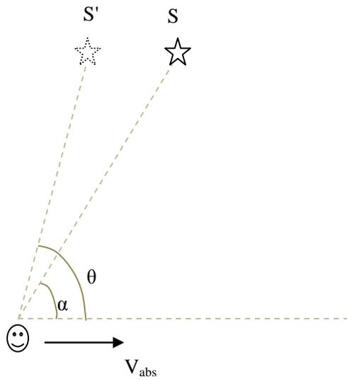
The quantitative expression of the angle of aberration for a star directly overhead is determined as follows [1].
