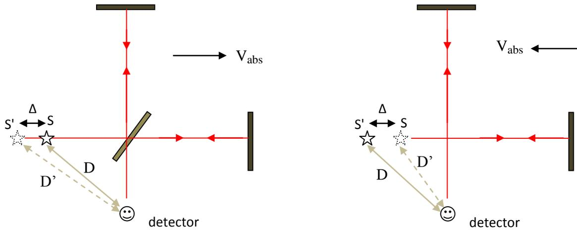
If the absolute velocity is directed downwards, as shown below, there will be an apparent change of source position in the upward direction. In this case there will be a small fringe shift due to unequal path lengths of the red and blue 'virtual' light rays. This can explain the small fringe shifts observed in the Miller's repetitions of Michelson-Morley experiment.
