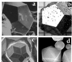
Fig 2: a.) Dodecahedral Quasicrystal Al65Cu20Fe15
