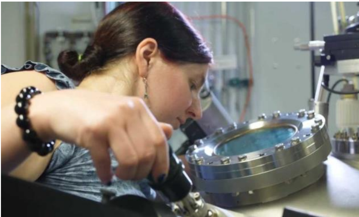
Jessica Steinlechner, one of the researchers, aligning a pulsed laser deposition system at Hamburg University to make an optical coating layer. Credit: Hamburg University
