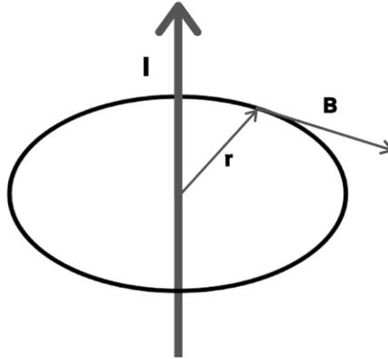
**Fig. 4:** Electromagnetic induction.  $I$  = current,  $B$  = magnetic induction intensity,  $r$  = radius of circle surrounding the electric flow line.
