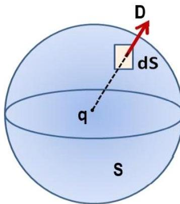
**Fig. 5:** The displacement vector  $D$  is related to the electric field strength,  $E$ , on the surface of the sphere via the expression  $D = \varepsilon_0 E$ . The surface area of two spheres with the same radius will differ in Euclidean space and positively curved space – it will be smaller in the latter.
