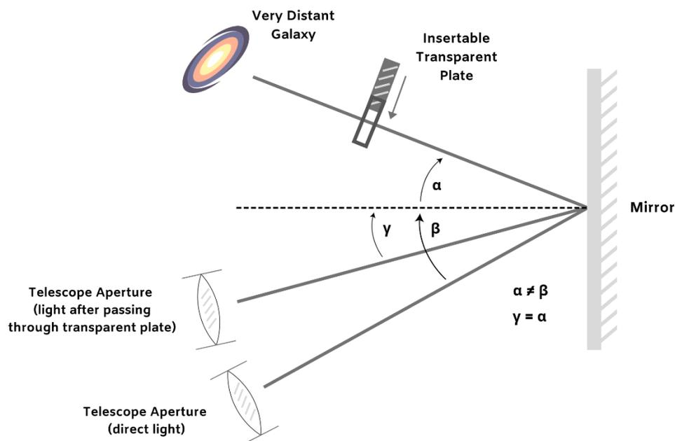
**Fig. 6:** Proposed experiment: a space telescope is set up to record images of distant galaxies indirectly – via light reflected from a flat mirror. The incident light is passed either through a transparent plate, or directly onto the mirror.
