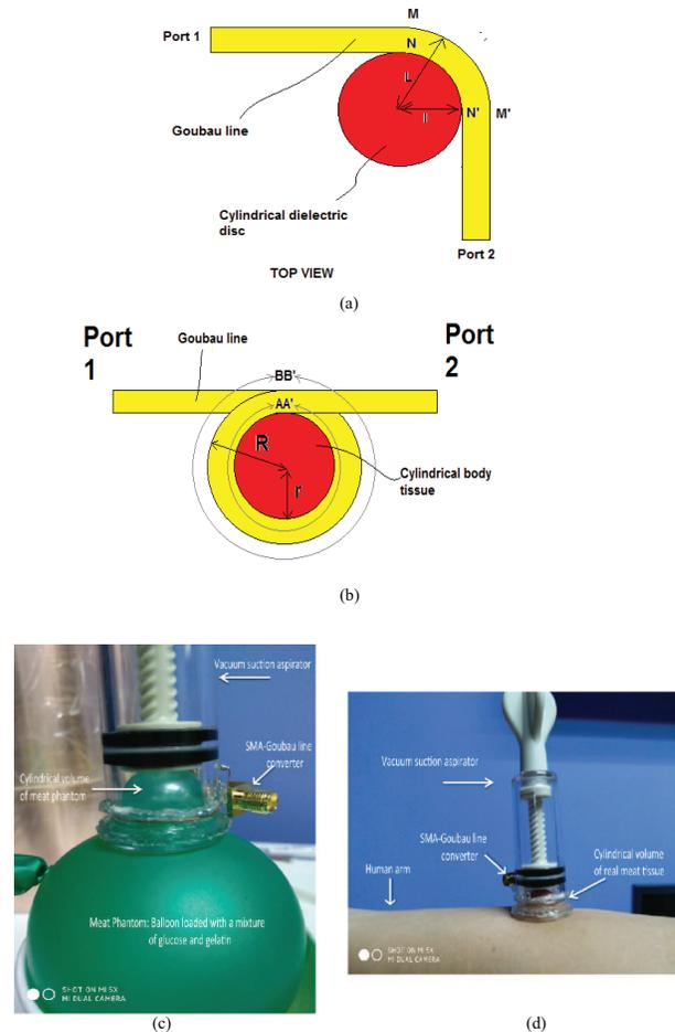
Fig. 1. Use of the dielectric cylinder for absorbing electromagnetic radiation. a) Original scheme proposed by Chiron for reducing radiation loss caused by the 90deg bend [7]; b) Extension of Chiron's scheme for measuring the dielectric constant; c) Suction aspirator for forming a fixed cylindrical volume of a meat phantom; d) Suction aspirator for forming a fixed cylindrical volume of a blood-filled human tissue.
