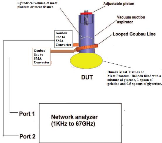
Fig. 2. Experimental setup for measuring blood glucose using a surface wave (frequency up to 67GHz).
