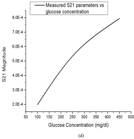
Fig. 3. S-parameters measured using Keysight Signal Analyzer N9030A: a) S21 parameters for frequencies from 1Hz to 67GHz; b) S21 parameters focused in the neighbourhood of 56 GHz; c) Measured S21 parameters as a function of Glucose Concentration.
