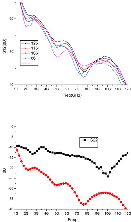
Fig. 4. S-parameters measured using Keysight Signal Analyzer N9030A: a) S12 parameters for different concentrations of blood glucose; b) S22/S12 parameters for blood glucose concentration at 109 mg/dl.
