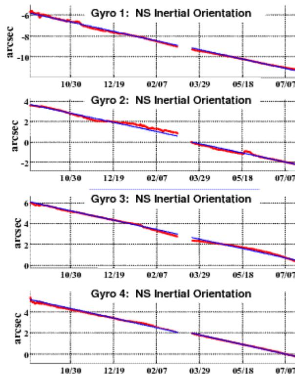
Graphs illustrate the changes in the size of the angle at which the axis of the gyroscope was located in the plane of the orbit of the probe, as time passes. So they show the direction of the axis gyro drift.
