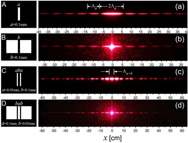
Figure 2: Comparison of diffraction and interference patterns between slits (Yin) and filaments (Yang), (a) single slit, (b) single filament, (c) double slit, and (d) double filament.
