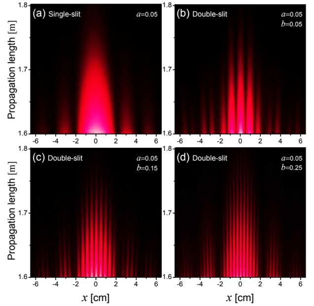
Figure 3: 3D diffraction and interference patterns of aquarium experiments, (a) single-slit of  $a = 0.05mm$ , (b)-(d) double-slit of  $a = 0.05mm$ ,  $b = 0.05mm$ ,  $0.15mm$  and  $0.25mm$ , respectively.
