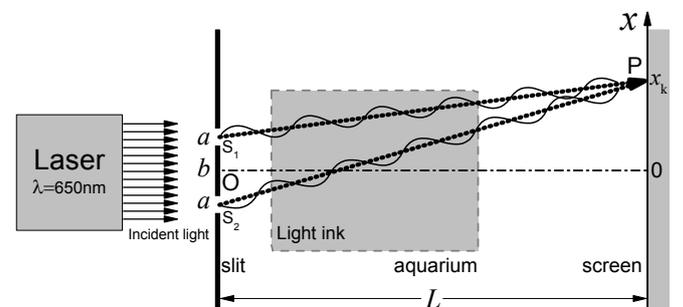
Figure 1: Schematic of improved Young's double-slit experiment.
