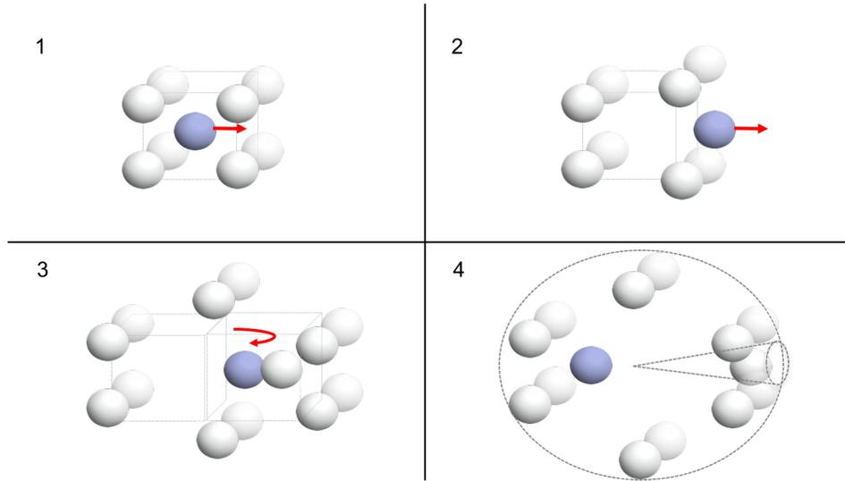
**Fig. 2 – Vibration of center granule in body centered cubic unit cell**
