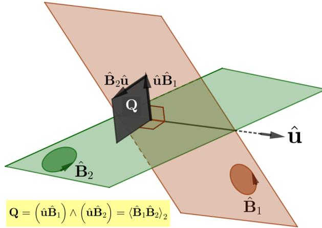
Figure 3: The bivector  $\mathbf{Q}$  contains (and is the outer product of) the vectors  $\hat{\mathbf{u}}\hat{\mathbf{B}}_1$  and  $\hat{\mathbf{B}}_2\hat{\mathbf{u}}$ . Although those two vectors are unit vectors,  $\mathbf{Q}$  is not necessarily a unit bivector, because the two vectors are not necessarily perpendicular to each other.
