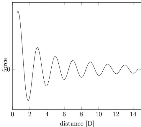
**FIG. 2:** Force between two standing waves.
