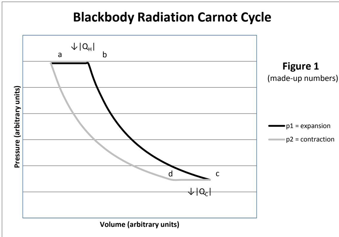
In figure 1, the lines drawn from points a to b, and from points c to d, are drawn greatly exaggerated, lengthwise, in this diagram. They should be drawn almost infinitely close to
