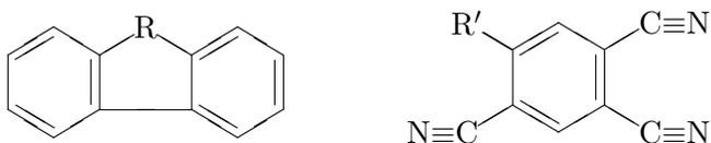
Figure 1. Left, N-Methyl Carbazole radical  $R$  denotes  $N^{\bullet\oplus} - CH_3$  abbreviated as  $NMCZ^{\bullet\oplus}$  and right Tetra Cyano Benzene radical with  $R'$  denoting  $C \equiv N^{\bullet\ominus}$ , abbreviated as  $TCNB^{\bullet\ominus}$ . In fact, the position of  $\oplus$  in the  $NMCZ$  radical and  $\ominus$  in the  $TCNB$  radical is unknown.
