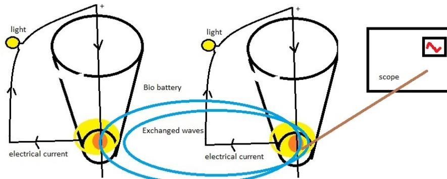
FIG. 11: A circuit of two shell less culture vessels (bio-batteries) and scope
