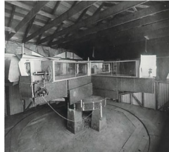
Fig. 0-11. Miller's Mt Wilson interferometer 41 .
