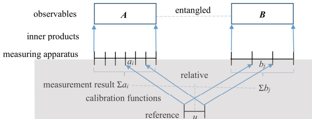
Fig. 1. Relative measurement system
