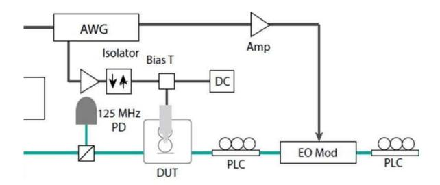
Extended experimental setup. The device is optically pumped by a tunable telecom laser centered around 1630 nm. The light is sent through an external electro-optic modulator and polarization controllers (PLC) before coupling into the chip ...more
