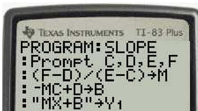
Figure 1: Code for linear regression using two points.
