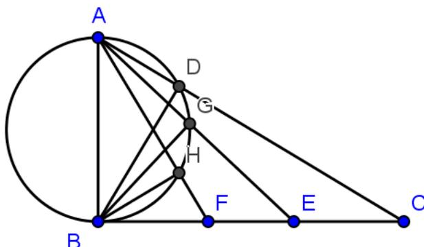
Fig. A3. Diagram showing equality of travel times along chords drawn from either extremity of the diameter of a circle in the vertical plane.
