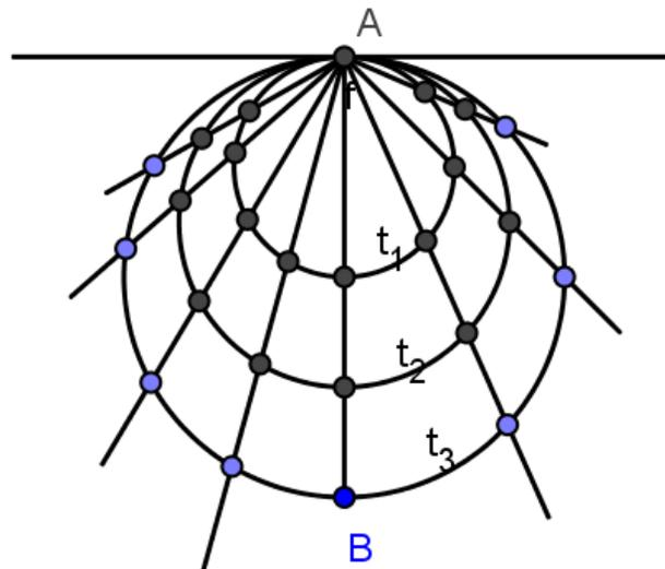
Fig. A1 Diagram showing that masses starting from rest from the upper extremity of a circle in the vertical plane travel any and every chord of a given circle in the same interval of time.
