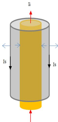
**Fig.1.** a cylinder conductor with current  $I_i$  is inside a long uniformly shell current of  $I_s$ . The two currents are in opposite direction. The blue arrows indicate the direction of the forces on the cylinder conductor and the outside shell.
