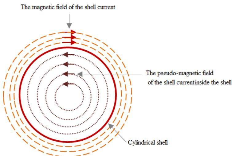
**Fig.2.** The cross section of a uniformly cylindrical shell current. The current flows into the paper.
