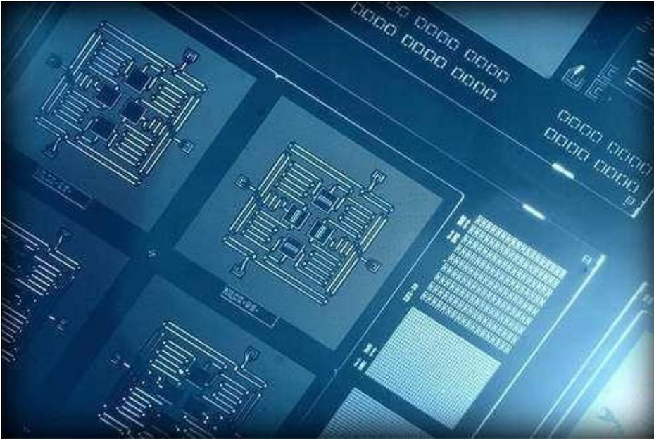
Layout of IBM's four superconducting quantum bit device. Using a square lattice, IBM is able to detect both types of quantum errors for the first time. This is the best configuration to add more qubits to scale to larger systems.
