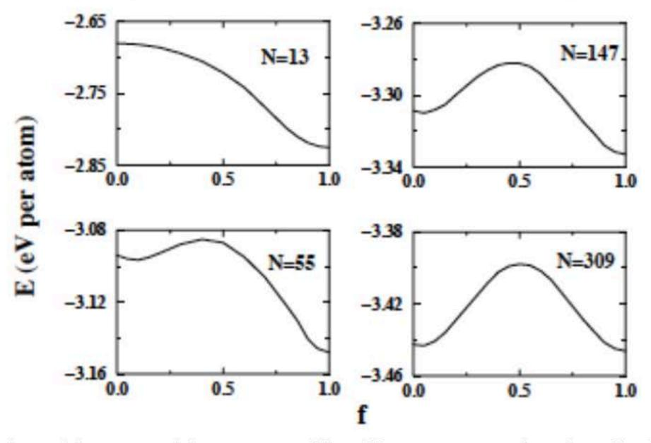
... The evolution of the potential energy profile of homogeneously relaxed ... PdN clusters during the Mackay [Jitterbug] transformation for increasing values of N. f is a fraction of the displacements ... f = 0 and 1 correspond to the ... cuboctahedron and icosahedron, respectively ...".
